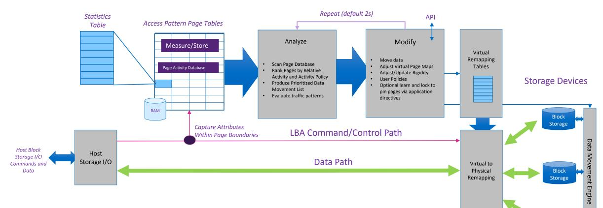
Goal of the engine is to continuously modify the virtual mapping until optimal performance is achieved using a policy driven model
